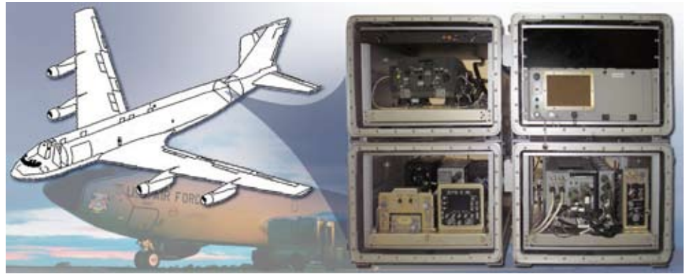
ROBE hardware provides rapid installation of a non-integrated TDL node for the KC-135 platform, and provides Link 16 LOS datalink support, BLOS gateway and SADL network support, chat and text messaging, user interface features, and FalconView and Gateway Manager (GM) situational awareness capabilities.
